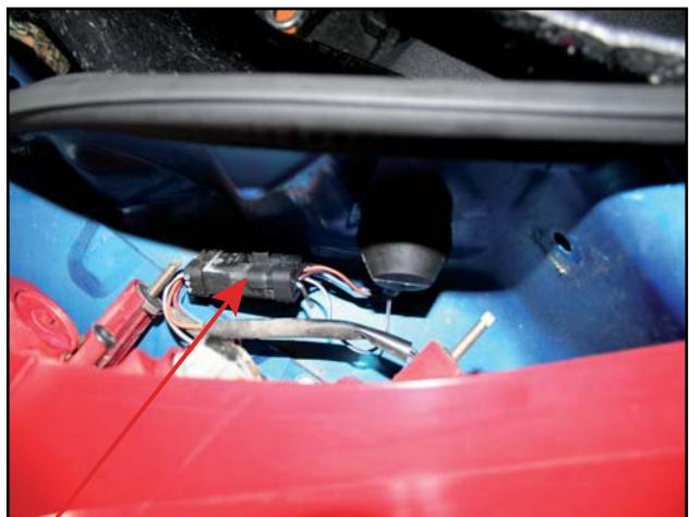
**Connector 6pin → 6pin Car**
